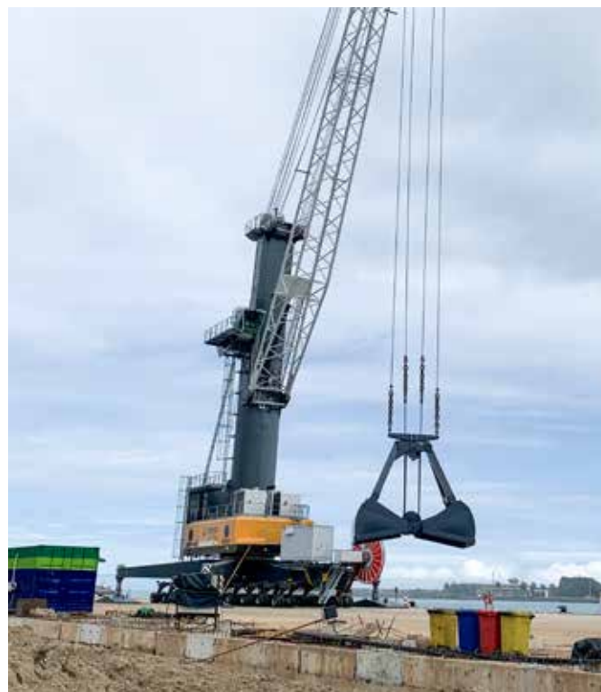
A HYBRID CRANE THAT CAN RUN ON BOTH DIESEL AND ELECTRICITY AT ARISE PORT TERMINAL, TIPSP, IN CÔTE D'IVOIRE
